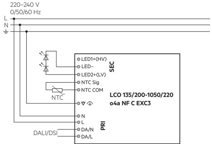
switchDIM with high voltage output (HV)
