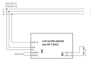
0/50/60 Hz Ν LCO 14/100-500/38 o4a NF C EXC3 N ⊕ L PR LED+ 0-● DA/N ヹ ⊕ DA/L switchDIM
