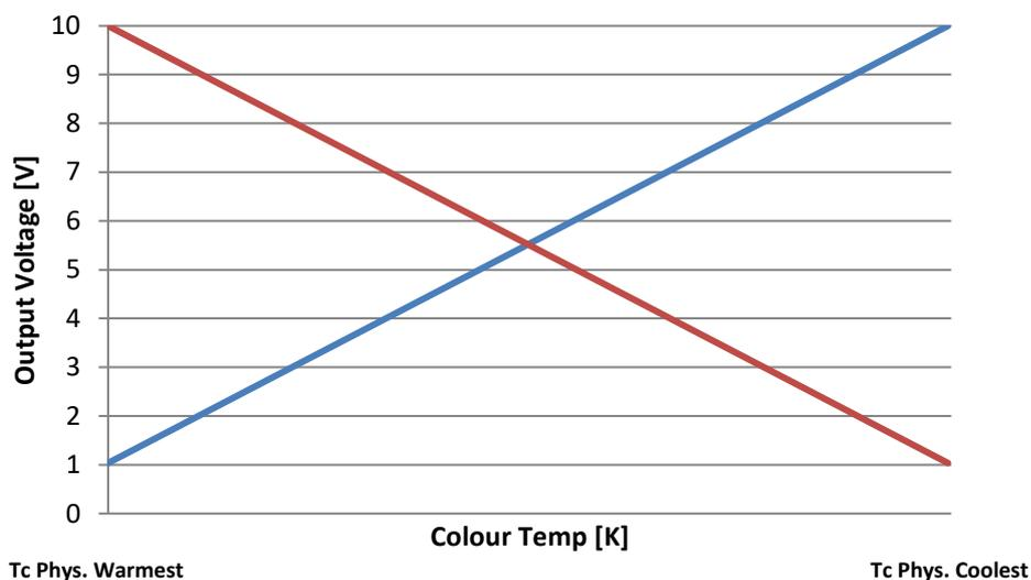
**Hint:** For a correct colour temperature the kelvin values of the used cold and warm luminaire should be entered as parameter TC PHYSICAL COOLEST and TC PHYSICAL WARMEST.
