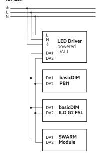
Single / free-standing luminaires, driver with separate power supply (DALI):
