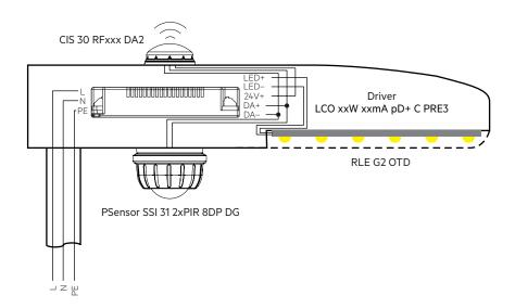
The sensor supports the Zhaga connectivity standard for Plug and Play luminaire extensions. This allows a toolless and flexible integration in luminaires. The connection interface is designed according to Zhaga Book 18 Ed. 3.
