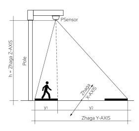
The detection range area y1 can be reduced if the sensor is mounted too close to the pole.
